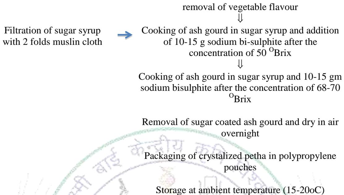
**Flow diagram for manufacture of 10 kg crystallized petha**
